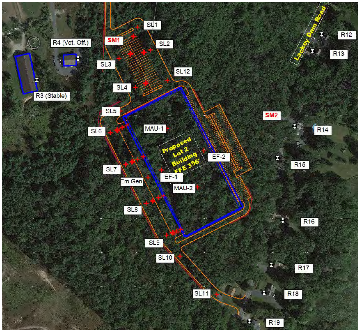
Figure 5. Stationary (MAU-1 & -2, EX-1 & -2, Em. Gen.) and mobile (SL1-SL12) sound source locations used in computer modeling Proposed Lackey Dam Logistics Center, Sutton, MA
