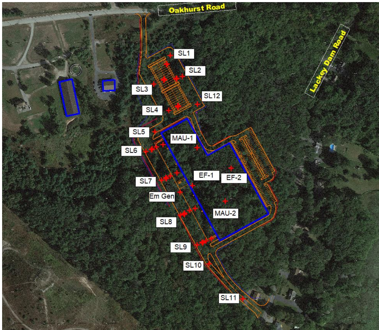
Figure 5. Stationary (MAU-1 & -2, EX-1 & -2, Em. Gen.) and mobile (SL1-SL12) sound source locations used in computer modeling Proposed Lackey Dam Logistics Center, Sutton, MA
