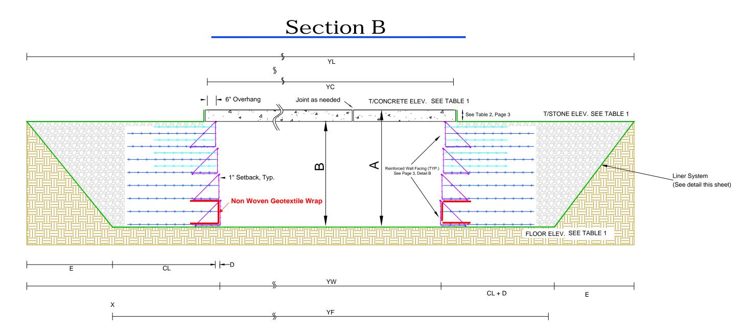
NOTE: AT THE CHAMBER END CAPS (14' WIDTHS), THE WALL SHALL BE CONSTRUCTED AS SHOWN IN THE BOTTOM 3 FT. OF OF DETAIL B, WITH 1 1/2" STONE, 9 INCH GEOGRID SPACING AND NO GEOTEXTILE WRAP.
